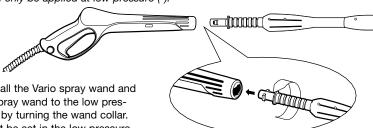
**Step 1** Install the Vario spray wand and set the Vario spray wand to the low pressure setting (-) by turning the wand collar. The wand must be set in the low pressure (-) position to apply detergents.
